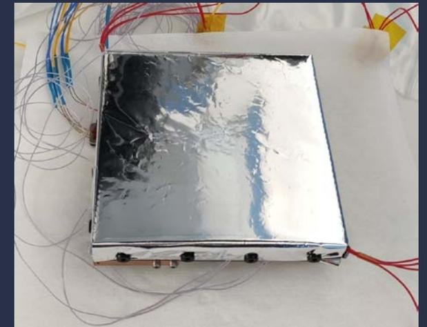
MLI attached to the thermal baseplate to minimise heat leakage
