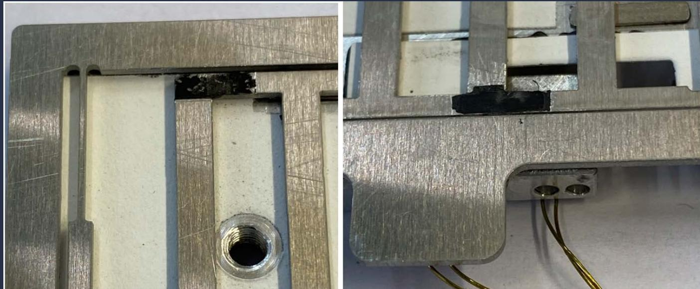
Missing spacer that fell off during vibration tests (top surface-bottom grid)
