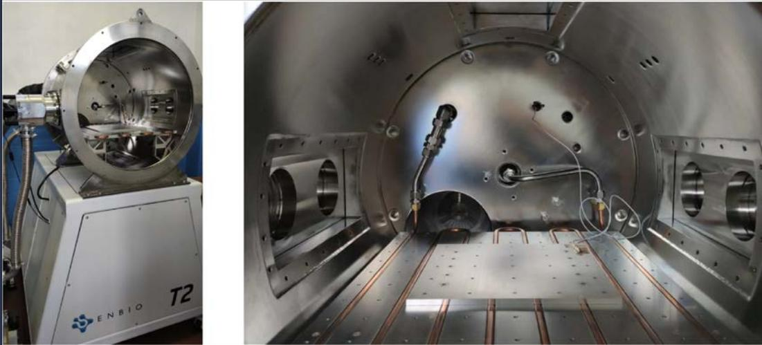
ENBIO T2 test facility used for thermal-vacuum cycling testing
