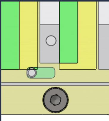
Inspection at CSEM after FOTEC tests determined the source being friction between the flexible grids due to detached spacers (see slide 67).
