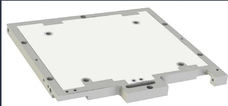
Baseplate with SolarWhite and masking pattern
