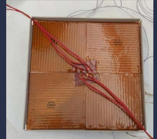
Kapton foil heaters attached to baseplate
