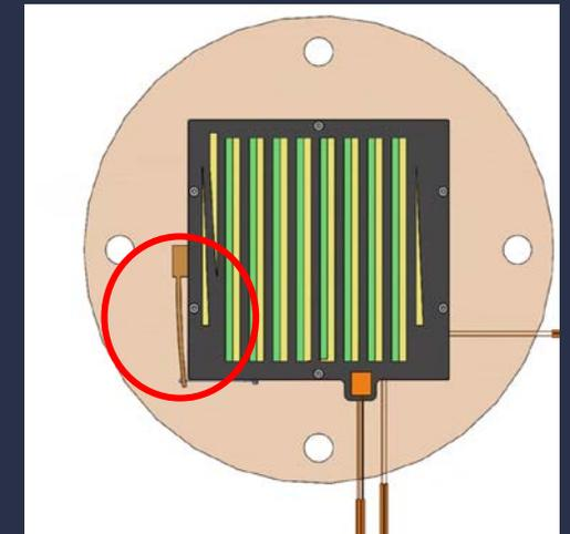
With spring-loaded dummy LLD
