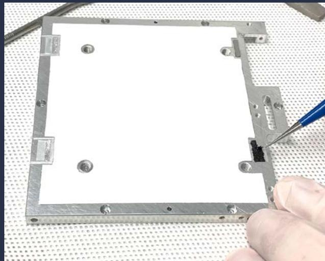
Removal of tape around epoxy and application of spacers
