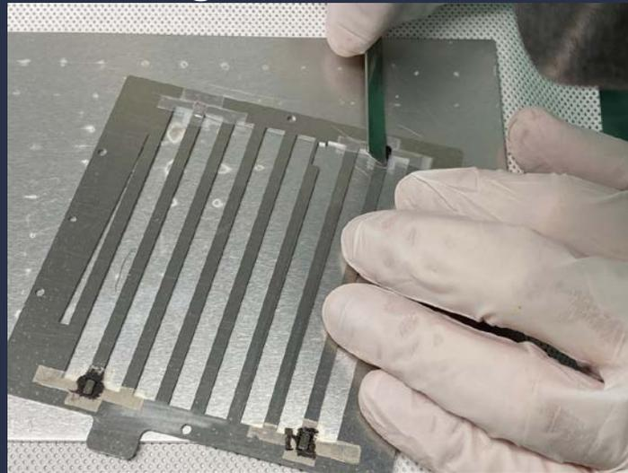
Application of spacer on epoxy
