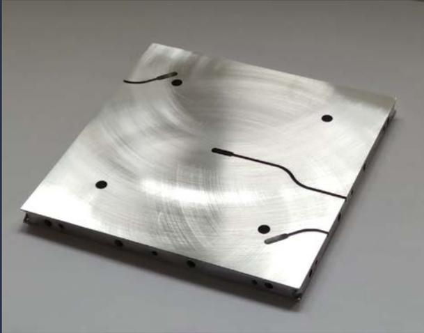
6 type E thermocouples embedded in the baseplate
