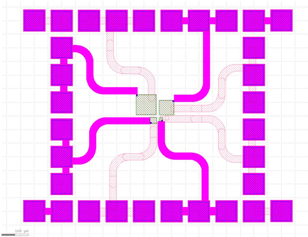
Figure 3: proposed single pixel test chip design incorporating four different pixel designs
