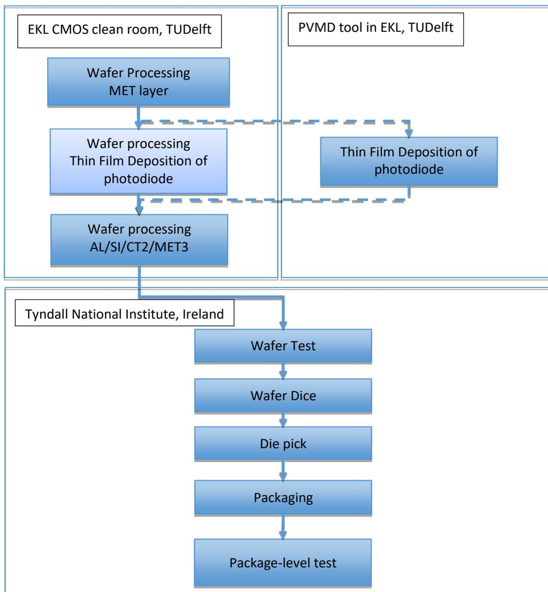
Figure 2: work flow of end-to-end manufacturing
