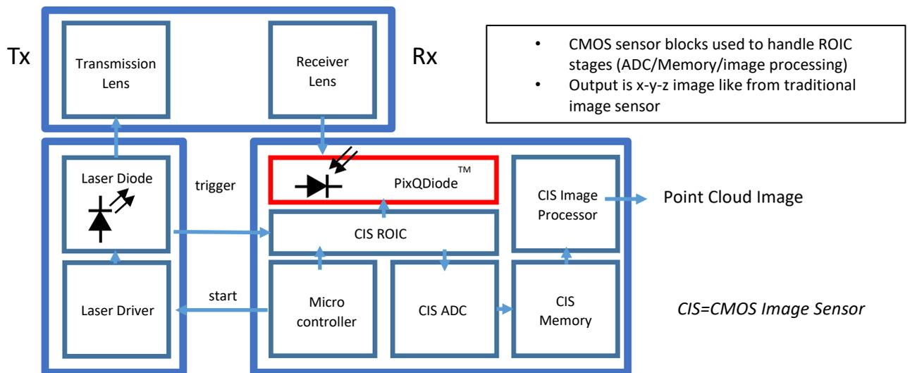
Figure 2: The LiDAR system concept as proposed, using a CMOS Image Sensor as the ROIC for a flash-LiDAR implementation
