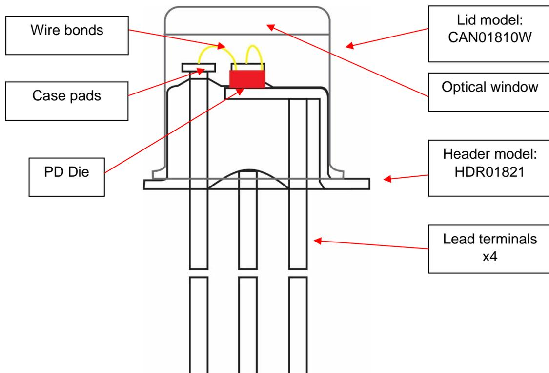
Figure 4: Cross section of TO18 package assembly
