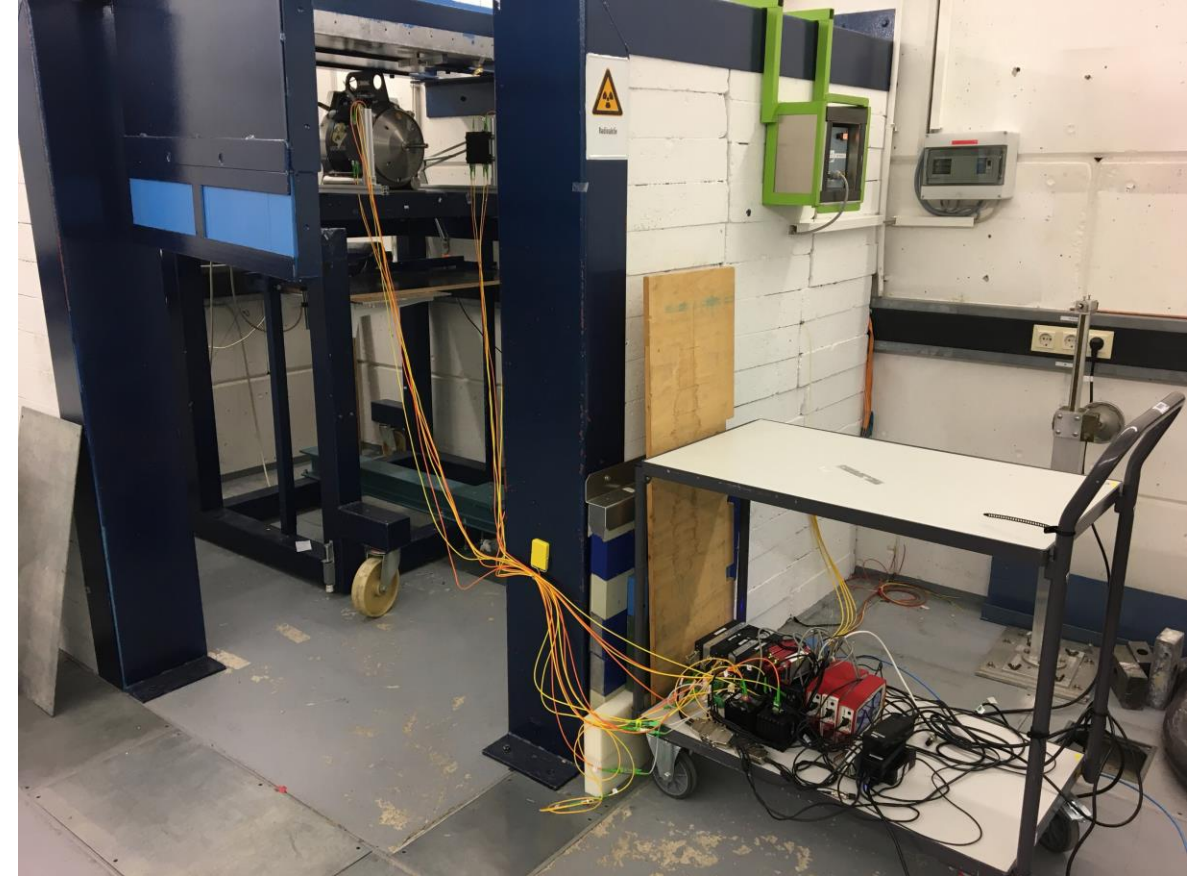
Laser controls behind lead shield
