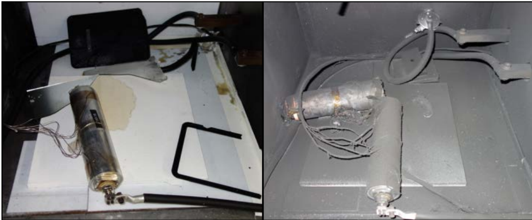
Figure 4-1: Pictures of two VES140 battery cells after external short-circuit test
