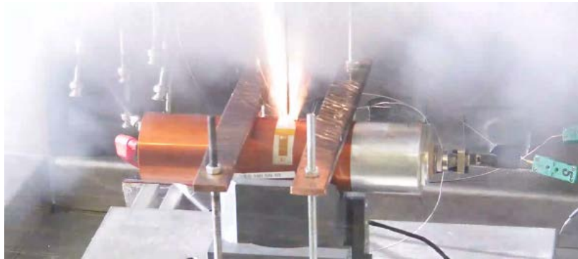
Figure 5-2: Picture of a VES180 battery cell before, during and after internal short-circuit
