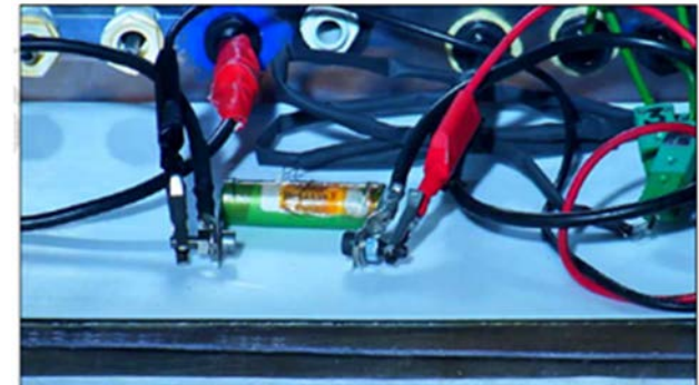
100 mΩ short-circuit on HCM cell
