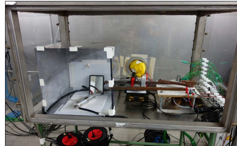
3 mΩ short-circuit on VES140 Test setup
