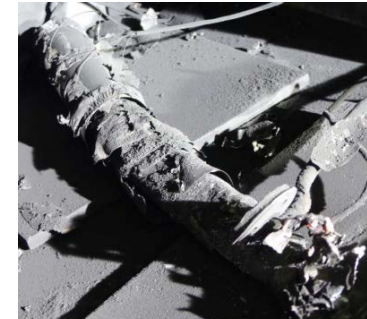
Overcharge at 2C - SOC at CID activation
