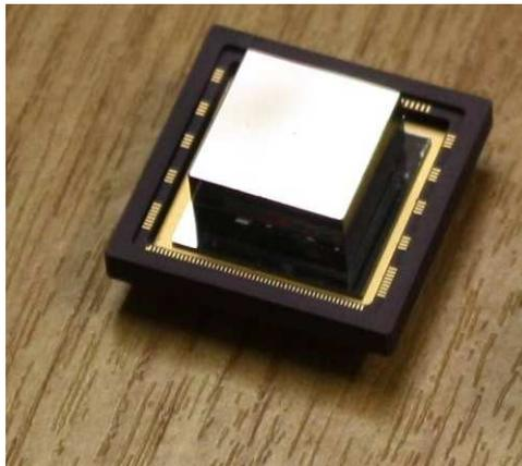
Figure 2.1-8: Mock-up integrated chip in package
