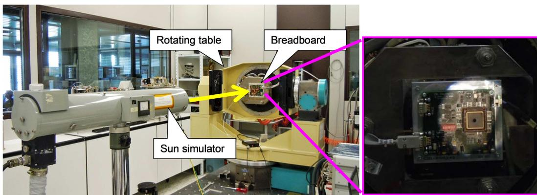
*Figure 2.2-2 SSoC prototype on the testing facility*
