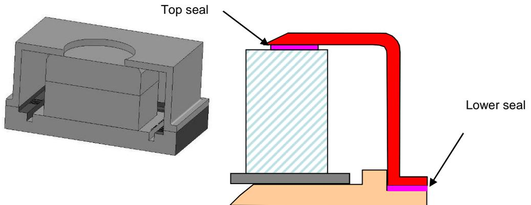
Figure 2.1-7: Section through package (left), Top and lower seals (right)
