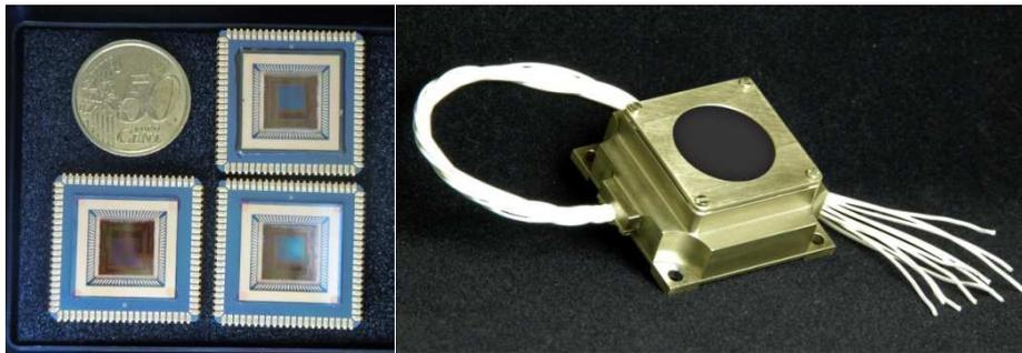
*Figure 2.1-1: First SSoC prototype in the standard package (left) and mechanical housing mockup (right)*
