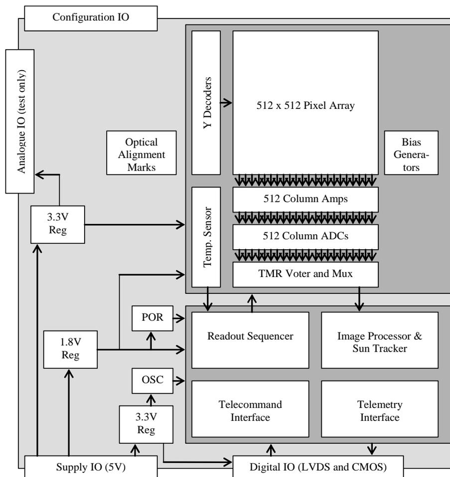
Figure 2.1-5: Sensor chip block diagram
