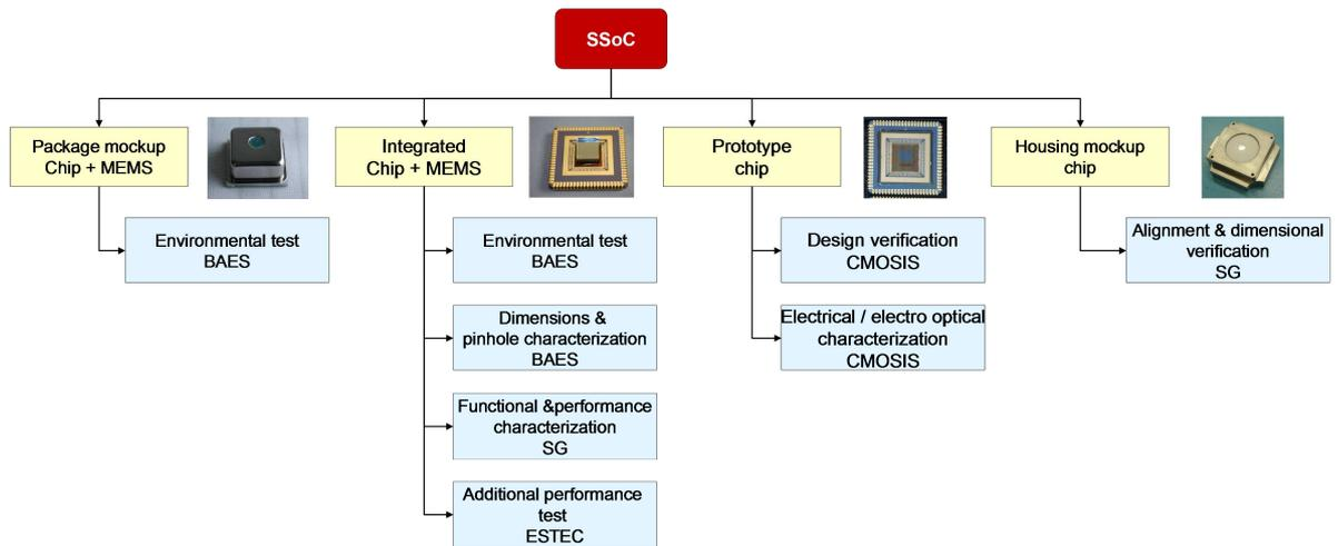
Figure 2.2-1 prototype samples testing activities
