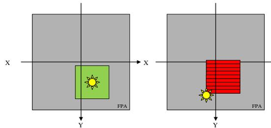
*Figure 2.1-2: Sun Tracking Mode with window scan: tracking (right), loss of Sun (right)*
