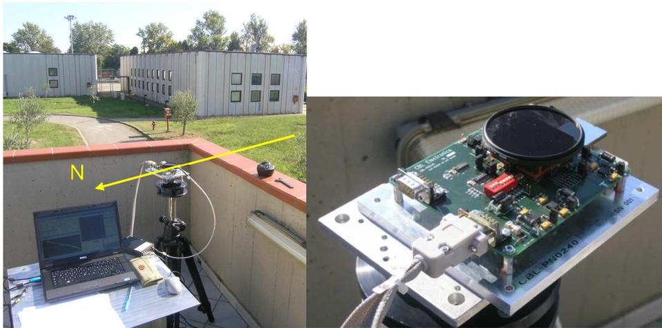
*Figure 2.2-3 Real Sun Test setup (left) - SSoC on the breadboard protected by ND filter (right)*
