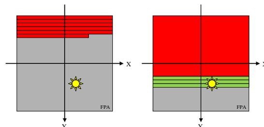
*Figure 2.1-1: Sun Acquisition Mode: full frame scan until the Sun image is detected*
