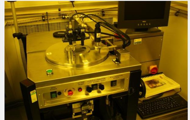
Equipment for wafer scale bonding
