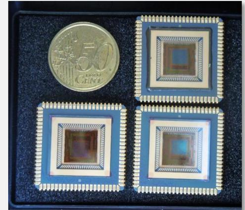
Prototype sensor chip in standard package
