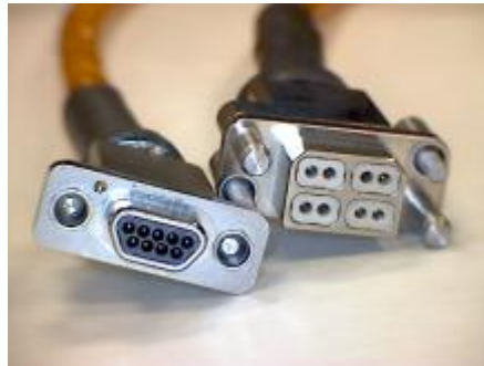
9 pin Micro-D connector versus MICROMACH®
