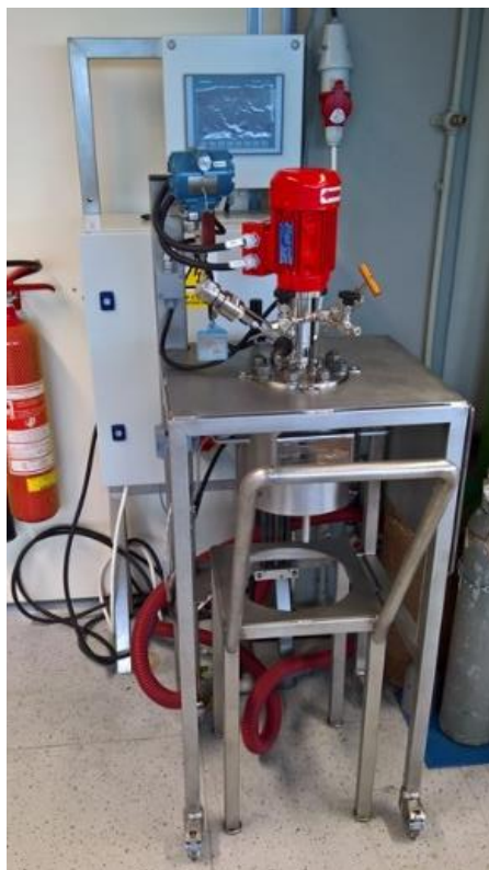
Photo of TOSEDA's laboratory pressure reactor set-up.
