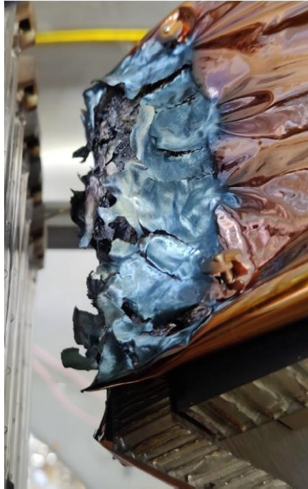
Figure 7-14: post-test damage of corner sample
