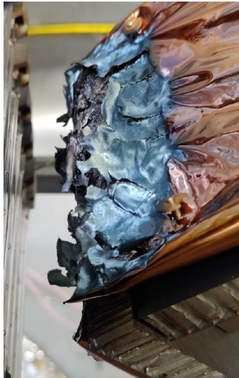
Figure 7-5: corner sample (with standoffs) post-static re-entry testing
