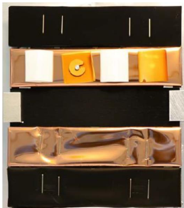
Figure 6-5: post-testing image of ATOX samples mounted to testing fixture
