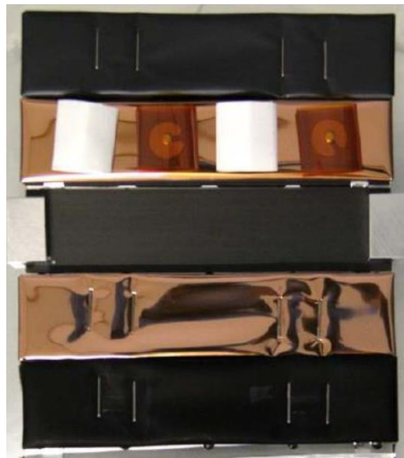
Figure 6-3: pre-testing image of ATOX samples mounted to testing fixture
