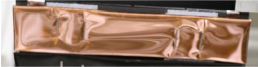
Figure 4-4: picture of ATOX MLI sample attached with Velcro
