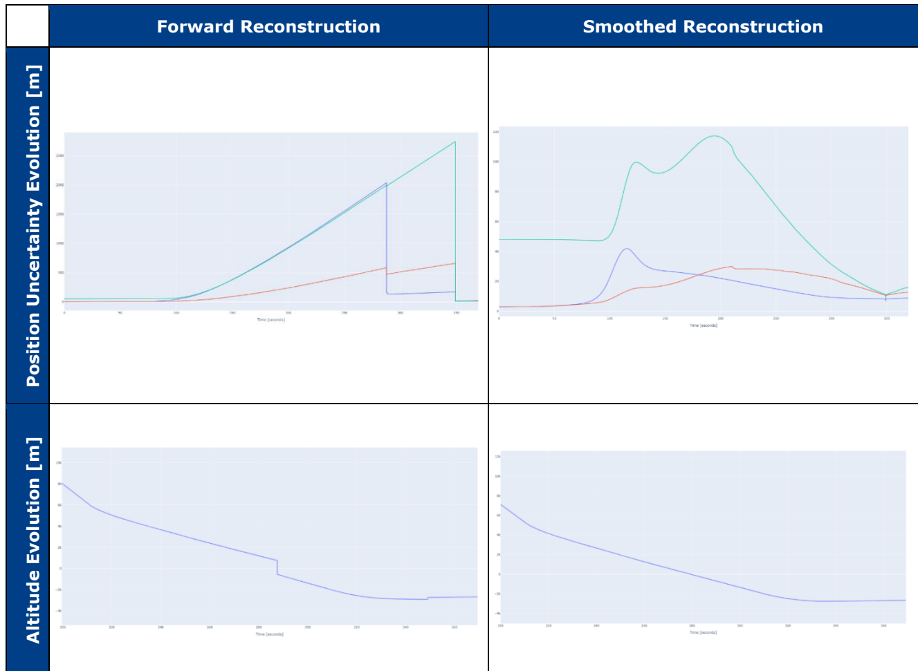
Figure 17: Forward (left) and Smoothed (Right) Position Uncertainty Evolution (Blue X, Red Y and Green Z Coordinates) and Altitude Evolution
