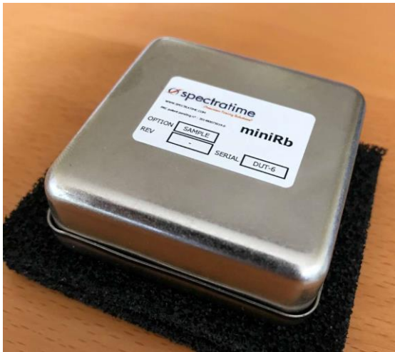
Figure 2.1: mTS clock unit (52x52x19 mm 3 )
