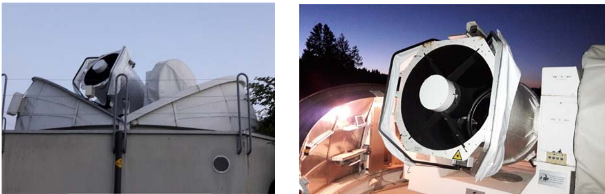
Figure 4-1: ZIMLAT telescope during the day when only SLR observations are used (left panel) and a closer look at ZIMLAT telescope during the night when CCD, sCMOS or simultaneous SLR and CMOS observations are used (right panel).
