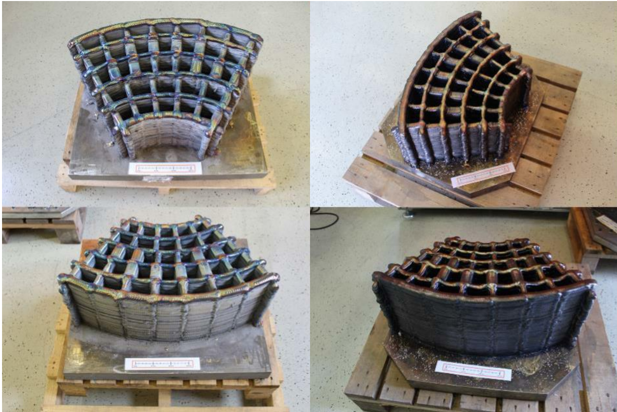
Figure 6. Finished Structural Model powder based (left) and wire based (right)
