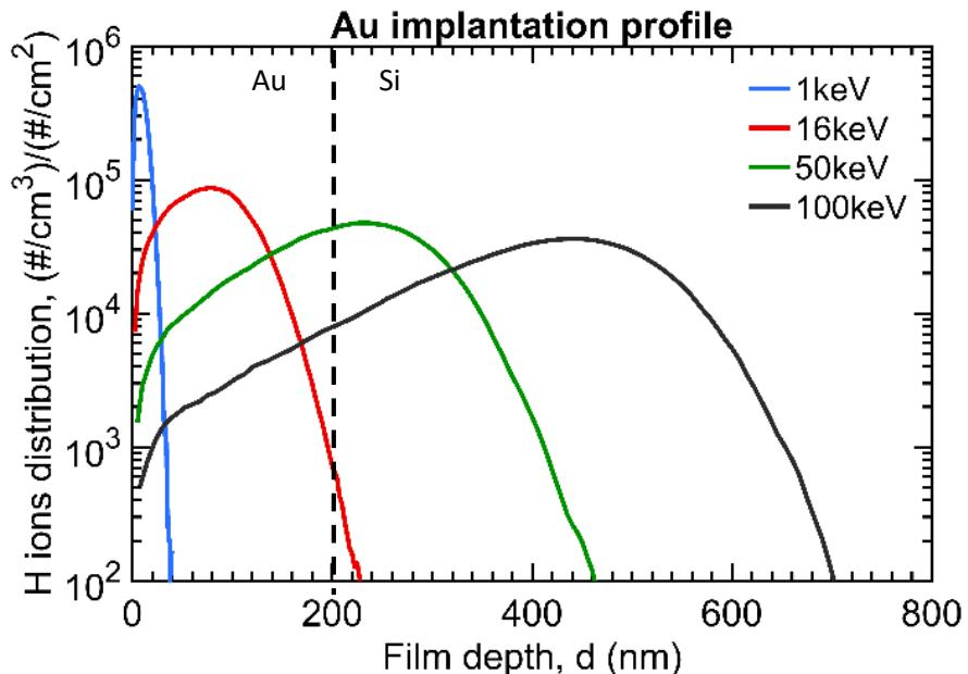
TRIM/SRIM simulations of the implanted protons distribution into bare and protected Al coatings for different energies.
