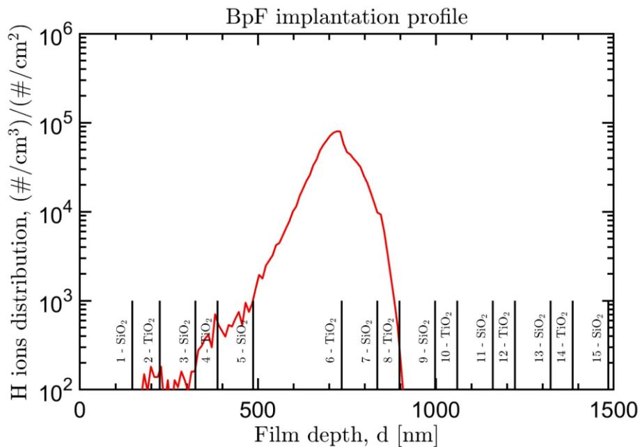
TRIM/SRIM simulations of the implanted protons distribution into a SiO<sub>2</sub>/TiO<sub>2</sub> band pass filter tuned at 590 nm (BpF) for a energy of 100 keV.
