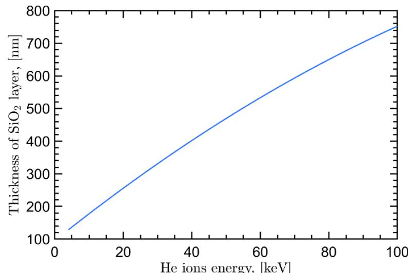
SiO<sub>2</sub> thickness required for stopping He ions at different energies. Data obtained from TRIM simulations.
