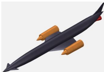
Figure 12: Concept Option 5 HSV with test propulsion components
