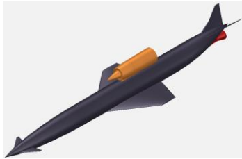
Figure 6: Concept Option 2 HSV with test propulsion components
