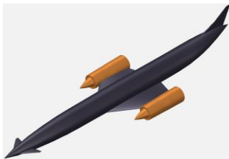
Figure 8: Concept Option 3 HSV with test propulsion components
