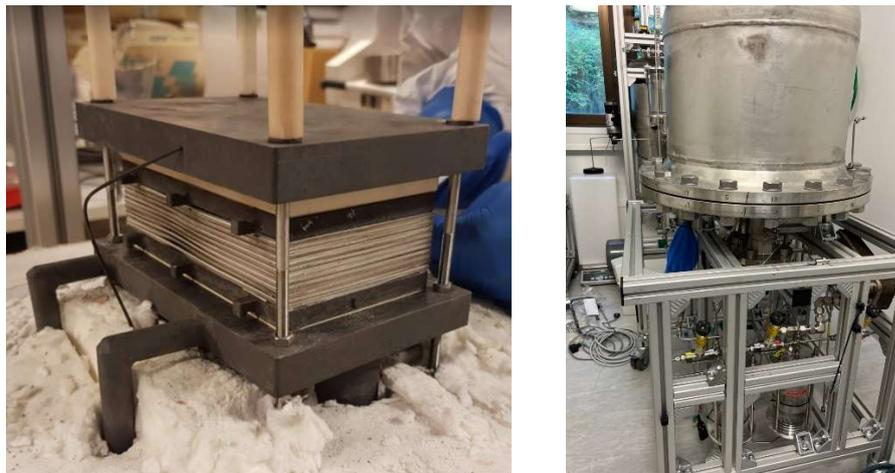
Figure 4. Left: Stack mounted on test rig. Right: Test rig for pressurised testing.
