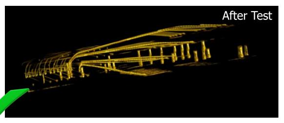
X-ray based 3D reconstruction of the GR740 bonds. Images courtesy of ST Microelectronics.
