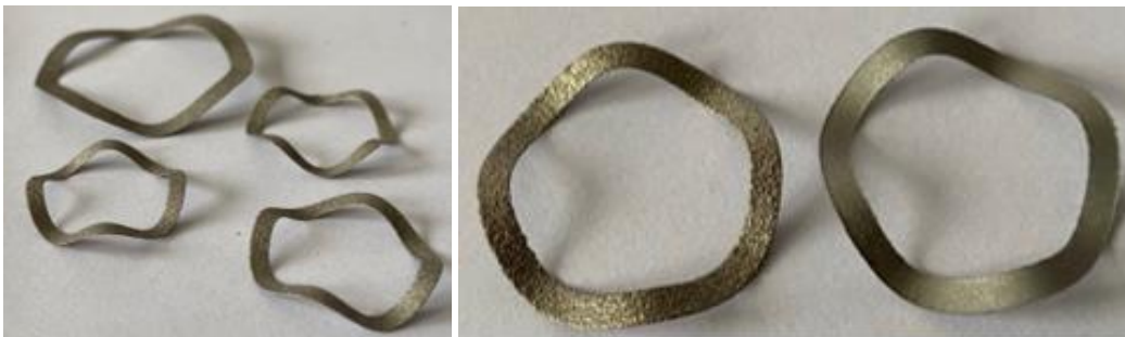
Figure 4 springs prepared by pmd via deposition of AMZ4 (left) and VIT105 (right) powders on alumina substrate.
