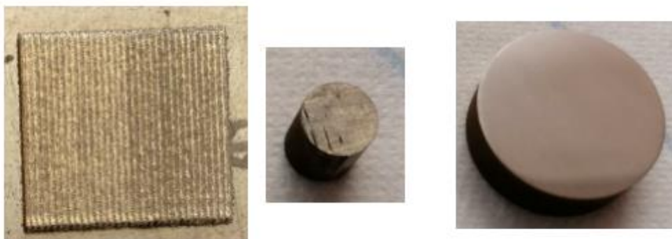
Figure 7 LMD deposited sample and machined set of pin and disc.
