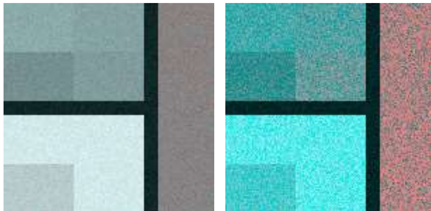
Figure 4-5: RGB color composite of monostatic HH (Red), monostatic VV (Green) and monostatic VV (Blue) on the left, and of bistatic VV (Red), monostatic VV (Green) and monostatic VV (Blue). Zenith incidence and scattering angle is 20^\circ and bistatic azimuth angle is 80^\circ . Stretching range is (-15 dB, 0 dB) for monostatic and (-30 dB, -5 dB) for bistatic.
