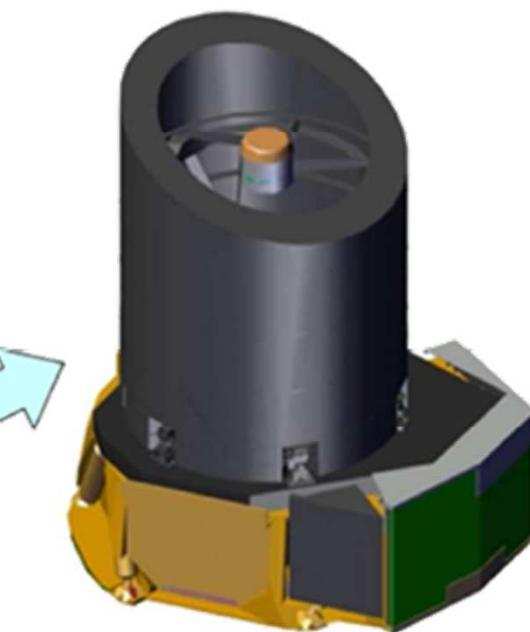
Payload Module (PLM), including the Telescope and the Optical Bench supporting the instrument detectors and front ends
