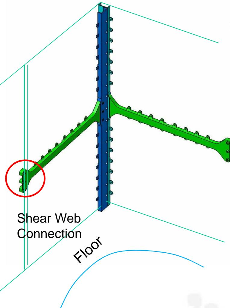
For the Frame Structure, **conical connections** guarantee accurate positioning of the parts and a high load transfer capability.
