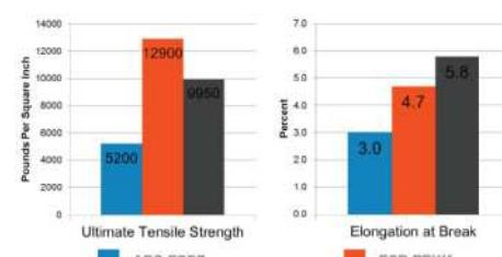
Figure 8 - Comparison of ABS-ESD7 and ULTEM 9085 resin to ESD PEKK in the on-edge build direction.
