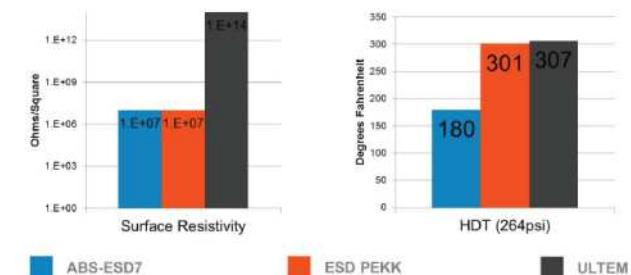
Figure 10 - Surface resistivity and heat deflection temperature comparisons between ABS-ESD7, ESD PEKK, and ULTEM 9085 resin.
