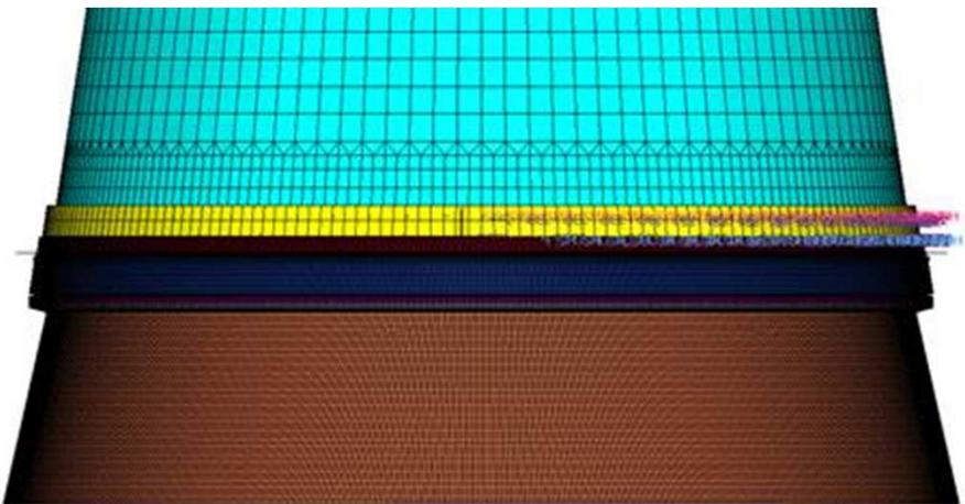
Simplified S3 FE on Adaptor; the Adaptor is clamped through RBE2 Spider
