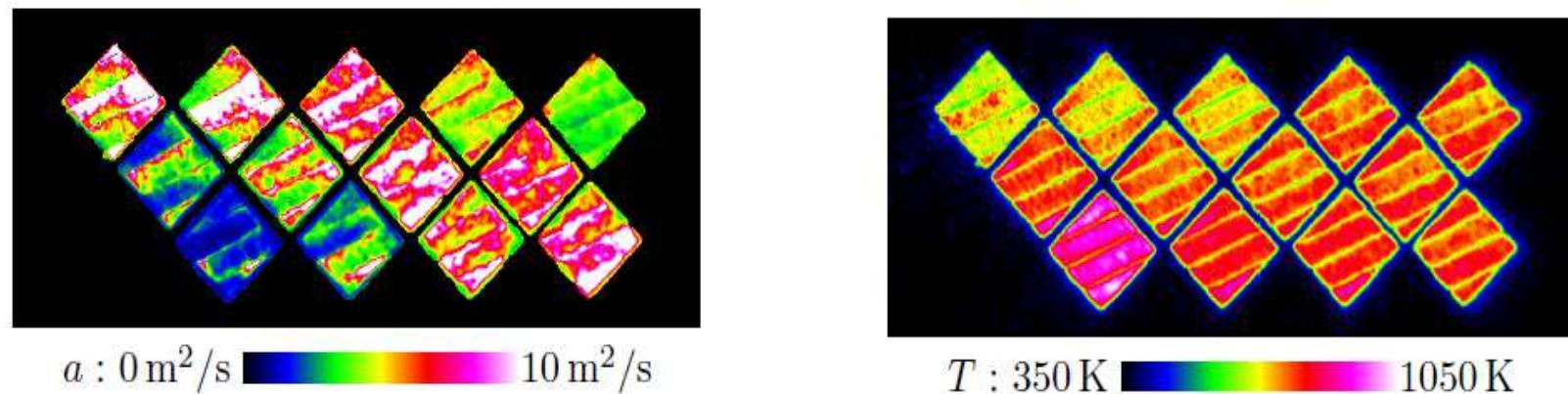
Fig. 4. Mapped key indicators for build height 3.6 mm: thermal diffusivity (left) and maximum measured temperature (right)
