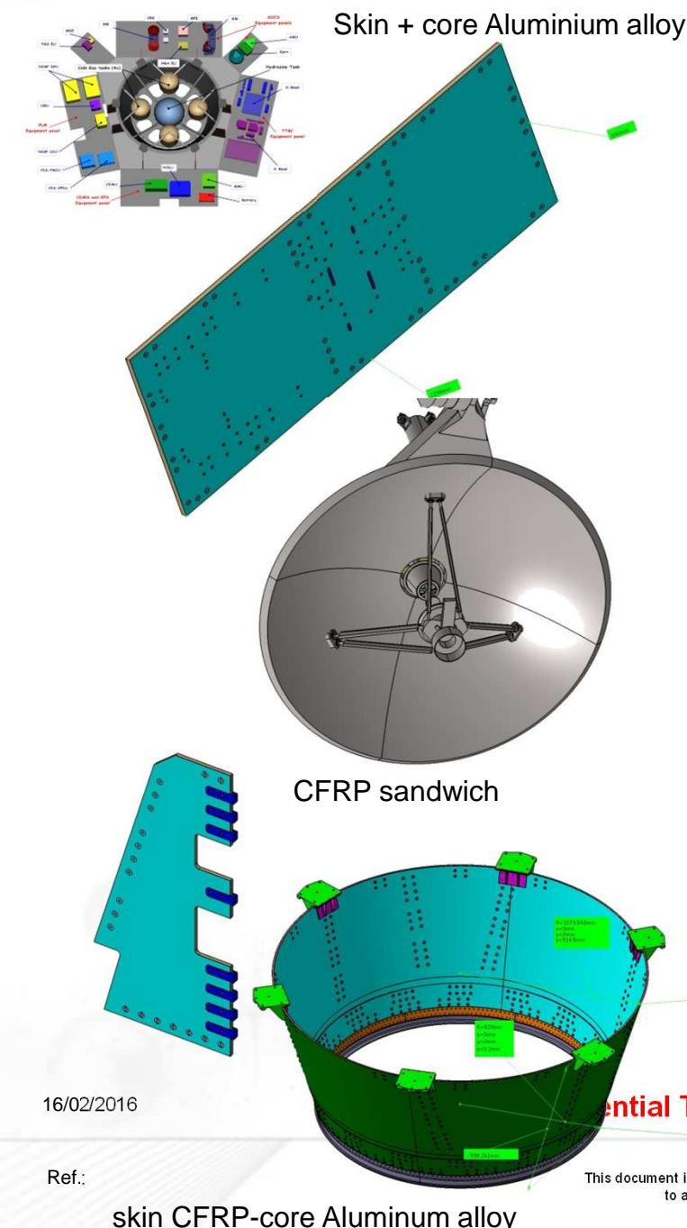
RUAG replaced the sandwich panel by aluminium frame:
