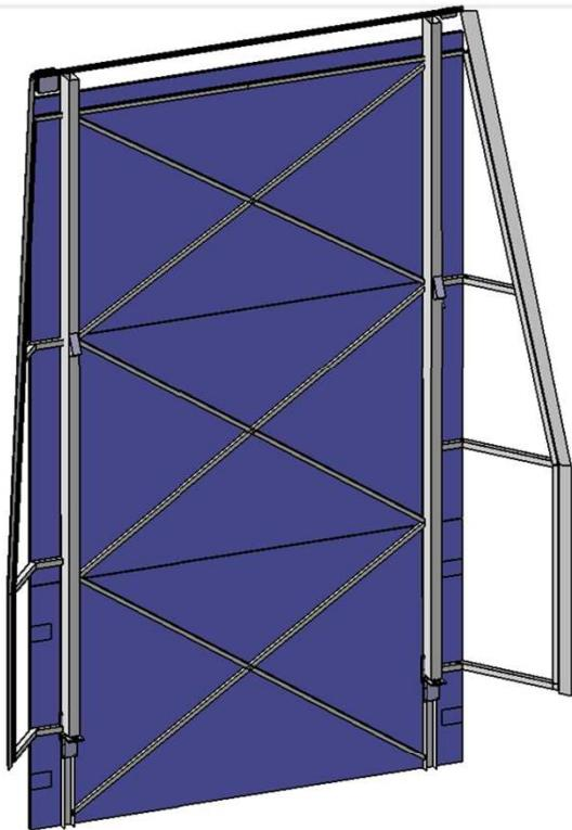
RUAG replaced the sandwich panel by aluminium frame
