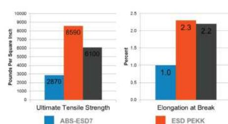
Figure 9 - Comparison between ABS-ESD7, ESD PEKK, and ULTEM 9085 resin mechanical properties in the vertical build direction.
