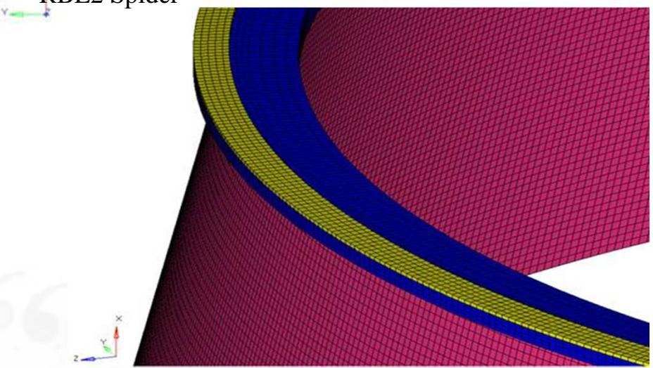
Yellow solid elements - contact area with the adaptor (merged contact nodes)
