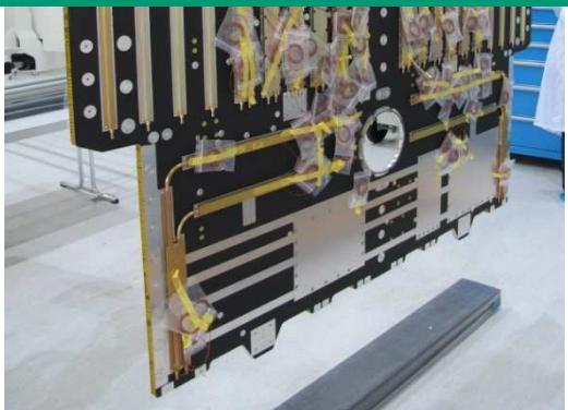
Heat pipe network on S GEO Payload Radiator
