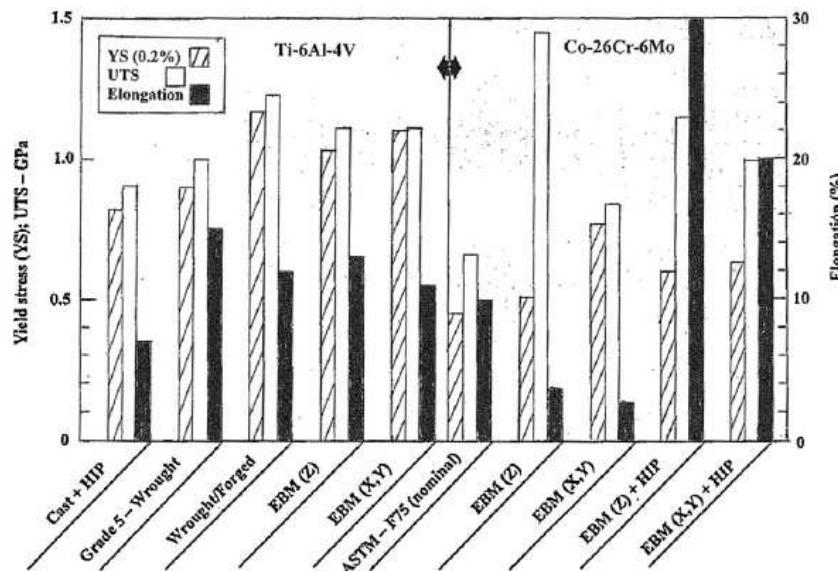
Fig. 15. Comparison of mechanical properties for commercial and EBM-fabricated and treated Ti-6Al-4V (left) and Co-Cr-Mo (Co-base superalloy). Commercial Co-Cr-Mo products are denoted by ASTM-F75 standard.
