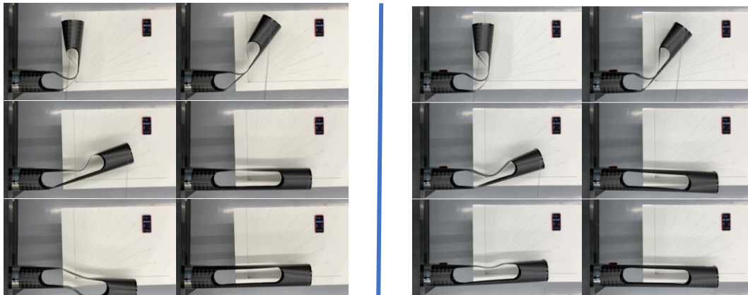
Figure 5. Loaded deployment sequence of the CFRP (L) and CFRFE(R) hinges (animations from left to right and top to bottom).
