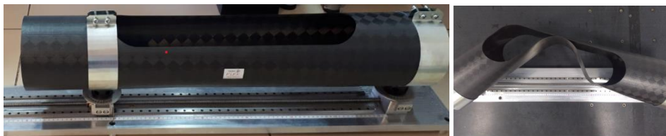
Figure 3. Demonstrator static characterization test: deployed position (L), during deployment (R).
