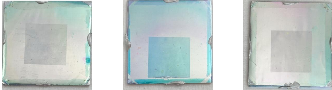
Figure 2: Test samples glued on Al 2 O 3 plates for testing. Size: 30 x 30 mm 2 ; pattern: 10 x 10 mm 2 .
