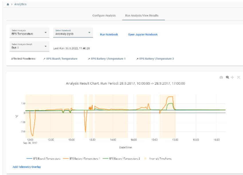
Figure 3 MachineLearning based anomaly detection results
