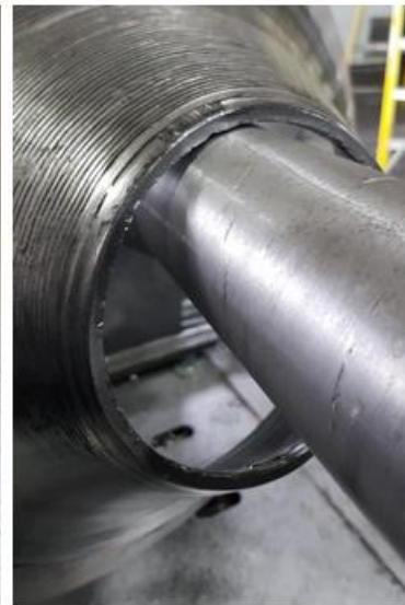
This resulted in endcap popping off 300mm into spinning process
