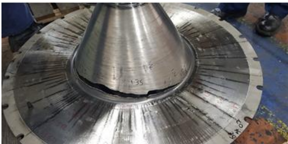
Circumferential ductile fracture failure
