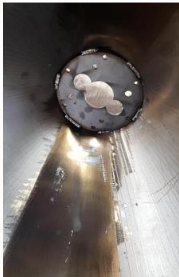
Tack welded on inside of endcap
