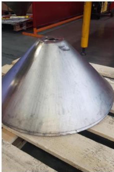
Part welded on side seams, Full penetration weld on outer endcap
