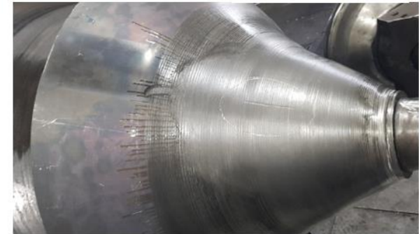
P4 weld seam crack failure 2
