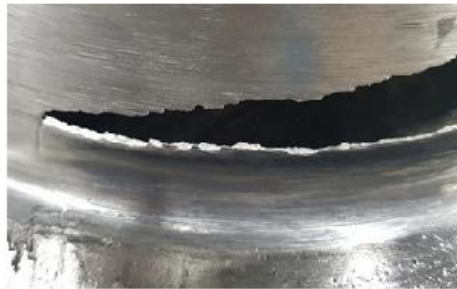
Close up of the left end of the crack propagation
