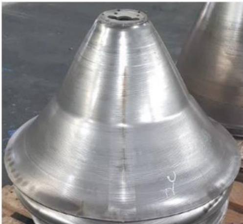
Project 3 (All failed - weld seam fracture)
