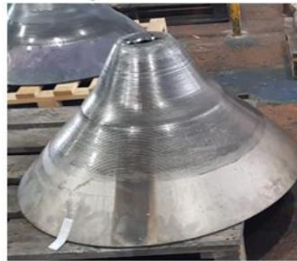
Project 4 (All failed, endcap and weld seam fractures)
