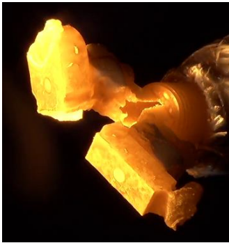
Figure 17: Melt of Head at Hole Location
