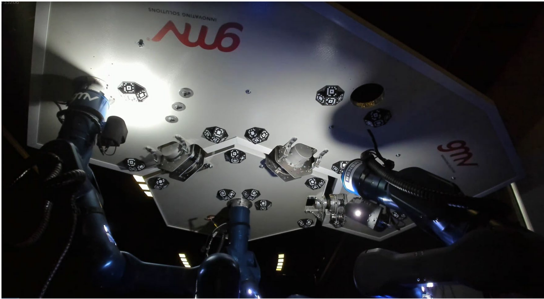
Figure 7-3 System vision robustness test in darkness
