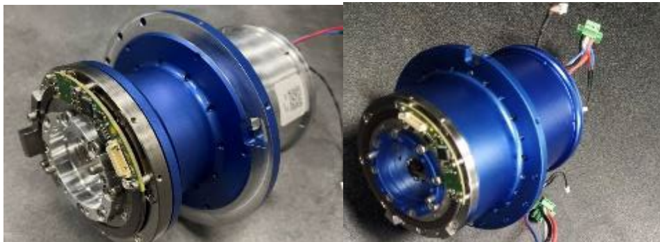
Figure 5-2: The two actuation modules "A" and "B" showing their main specifications and common mounting interfaces. At the bottom the two prototypes of size A and B drives.
