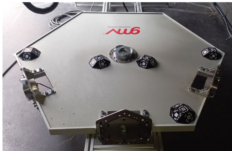
Figure 5-12: 3D arrangement of AprilTag markers on SMT mock-up
