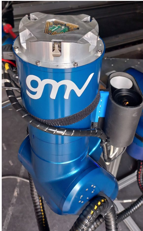
Figure 5-11: Optical head (camera, lens and light) mounted on one of the manipulators
