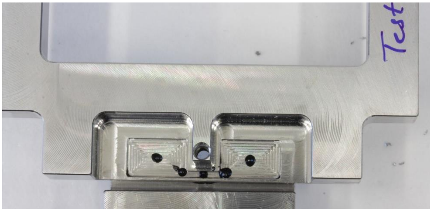
Figure 6 In-vacuum adhesive bonded sample
