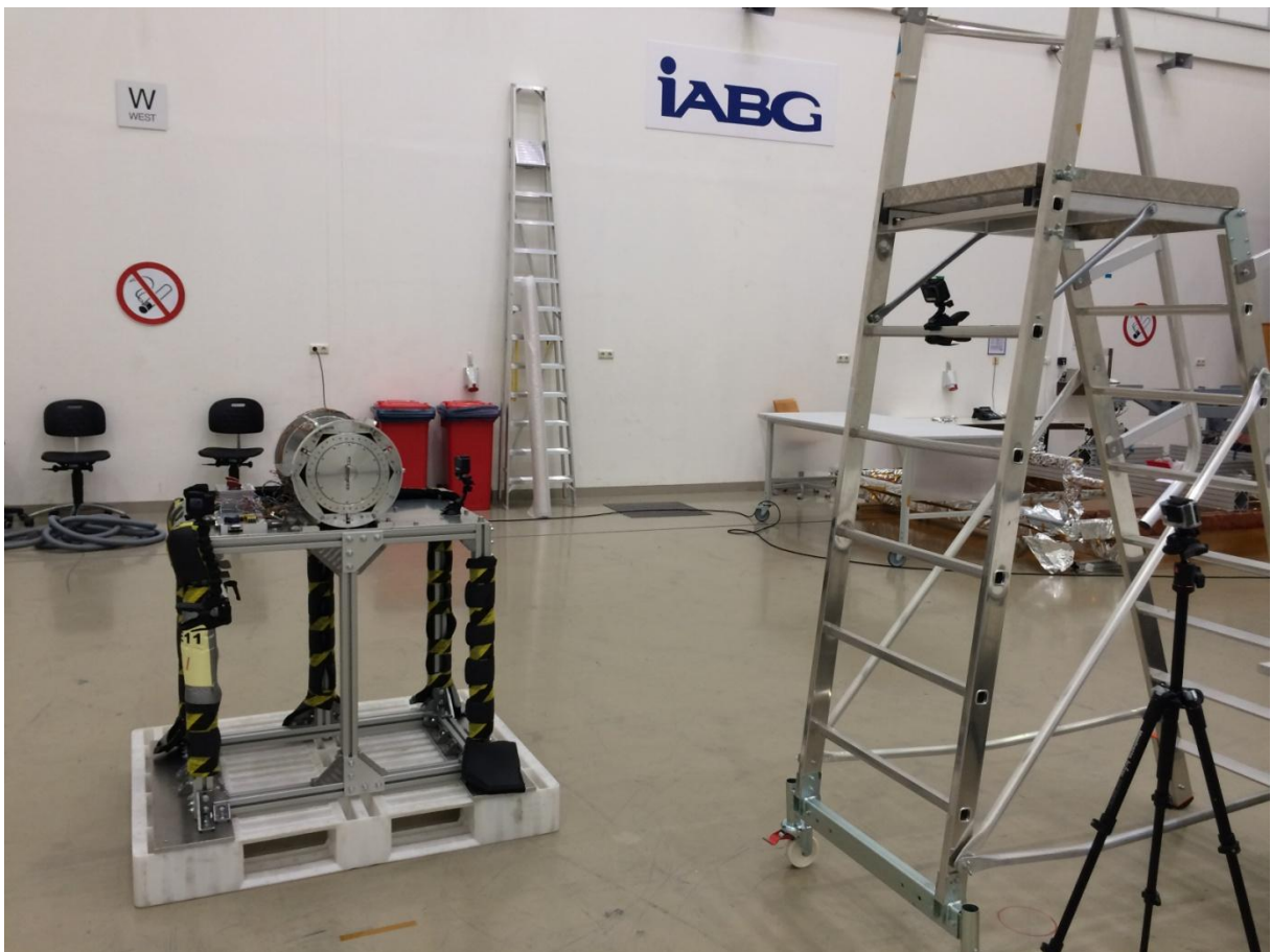
Figure 2-3: Test setup for ground deployment test, with ballute container and several cameras
