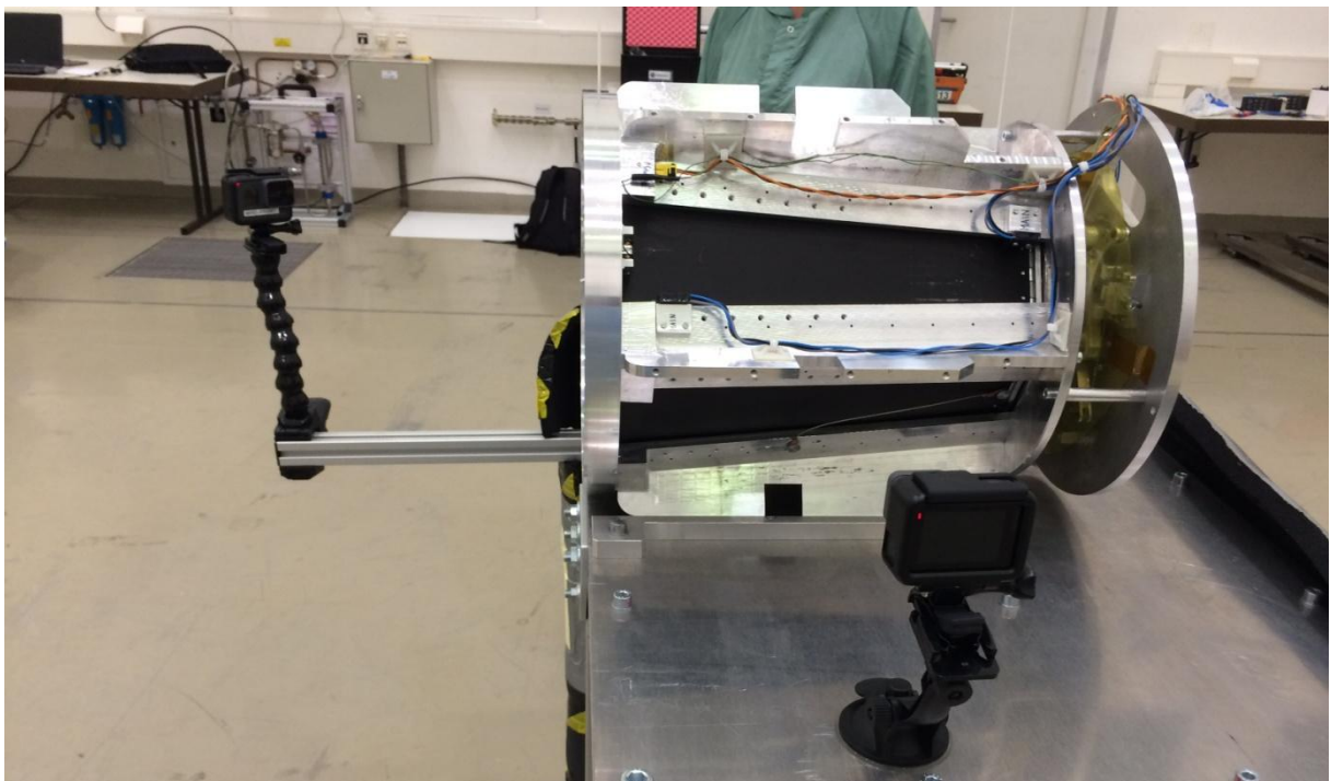
Figure 2-2: Ballute container on parabolic flight setup
