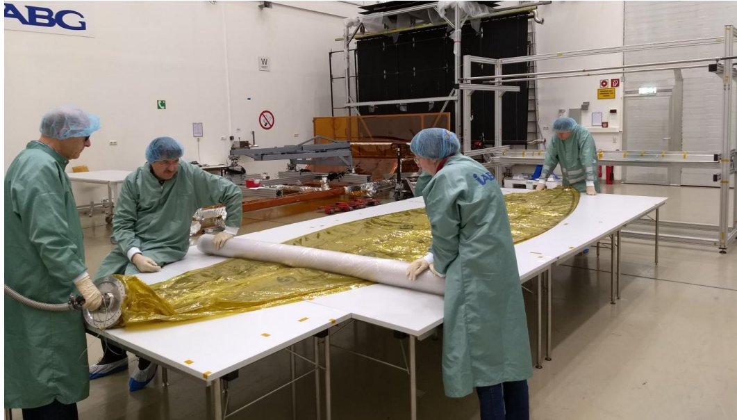
Figure 2-6: Evacuation of balloon (folding rig in the background)
