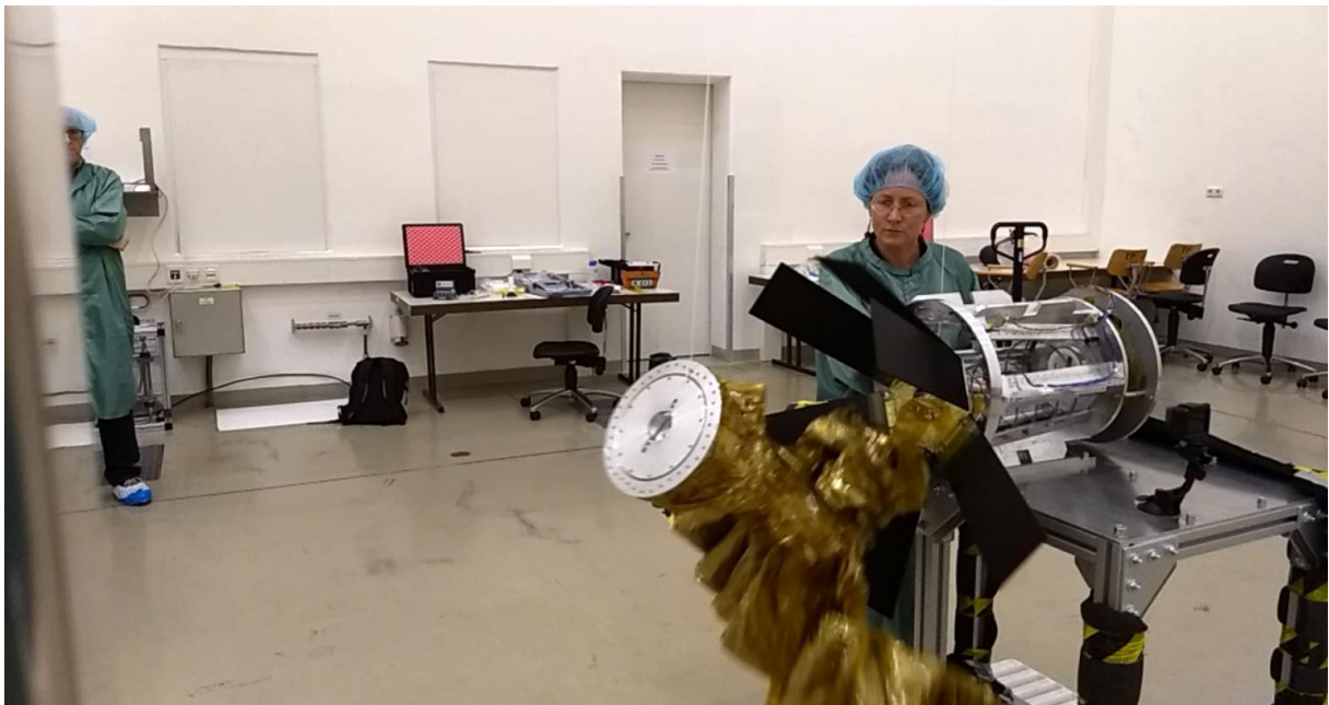
Figure 2-5: Final ground deployment test at IABG (still picture from video)
