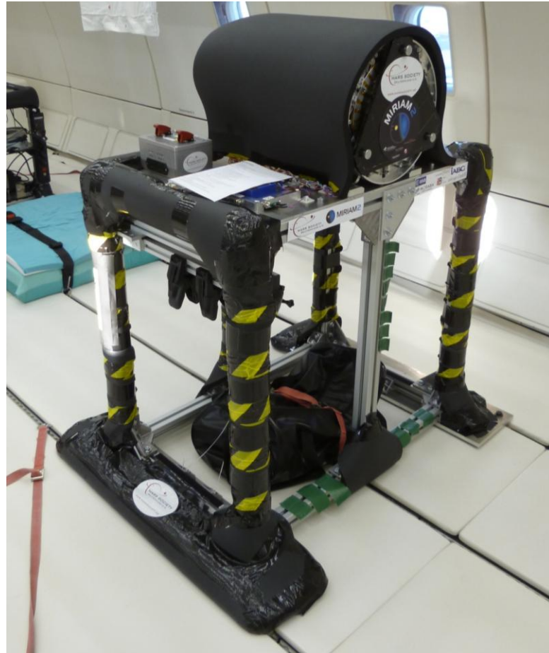
Figure 2-8: Test Setup in A310 Zero-G with protective covers
