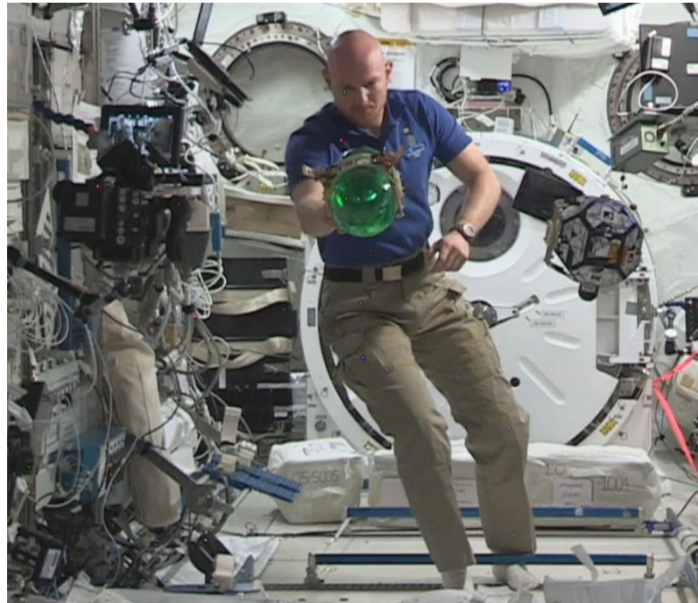
Figure 2: Astronaut Alexander Gerst disturbing the slosh tank (in green) with his finger during the fourth test session on October 18 th 2018.
