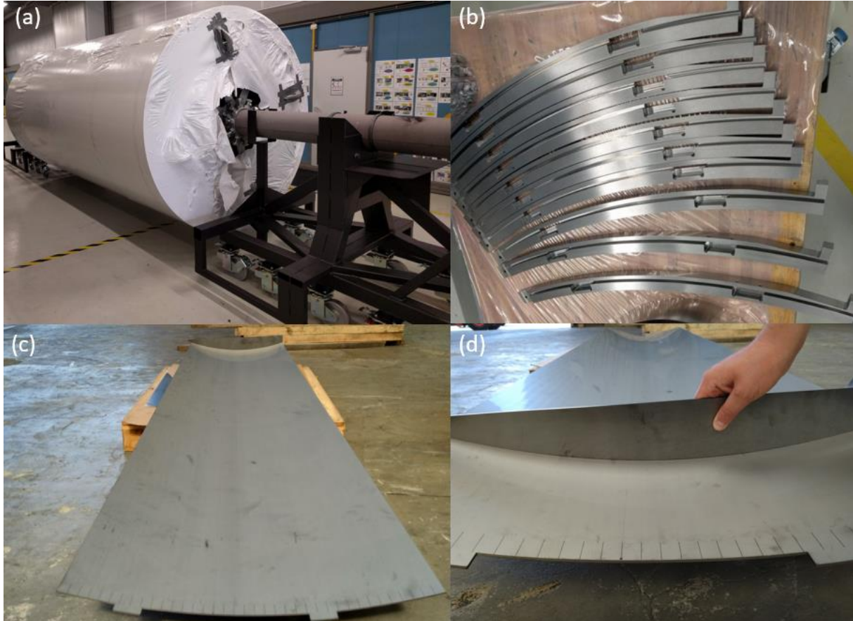
Figure 5 - Images showing (a) the mandrel and its support jigs, (b) edge dams, and (c) a caul plate, as well as (d) a dimensional check with a laser cut template.
