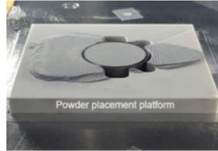
Powder spreading testbed (Lab-based test)
