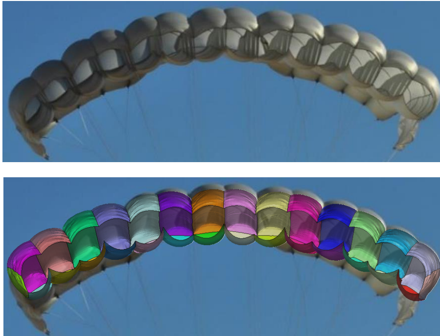
Figure 1: MC-4 canopy in flight (above) and overlaid with simulated inflated geometry (below)
