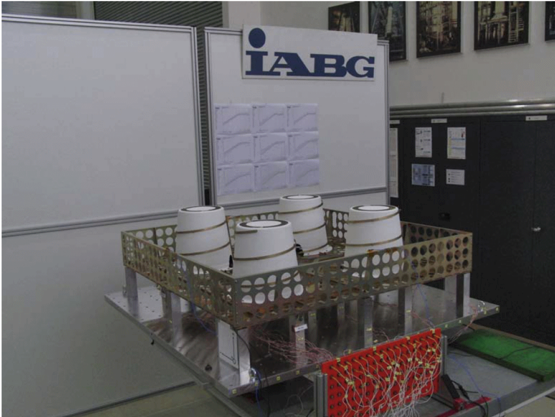
Figure 4.6.3.- Pyroshock testing set-up
