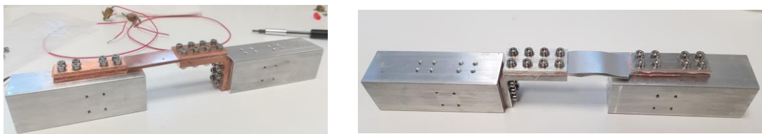
Figure 3-13 Copper and aluminium thermal straps mounted onto heat sinks
