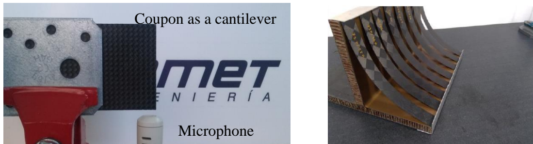
Figure 5. Damping test (L) and creep test (R) setups.
