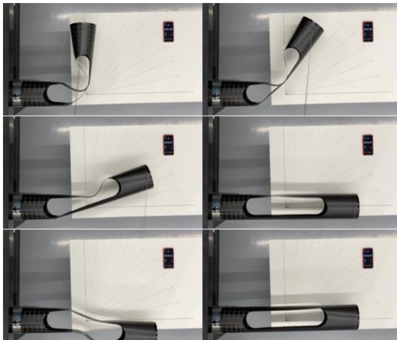
Figure 13. Loaded deployment sequence of the CFRP hinge (left to right and top to bottom).
