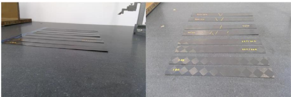
Figure 6. Flatness verification of creep coupons after cycling.
