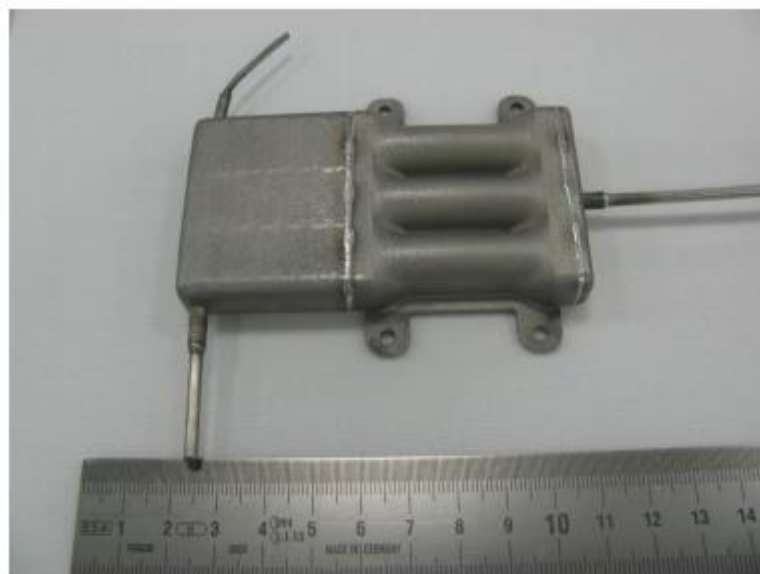
Figure 4: AM Flat LHP Evaporator - BBM
