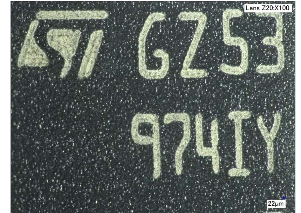
Examples of ST-Microelectronics Op-Amp Markings Following Solvent Tests (30X / 100X Mag)
