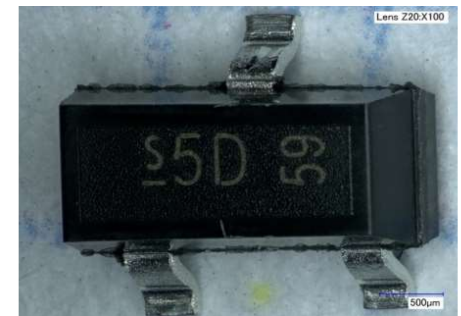
Infineon Diode – Marking “59” on oldest lot (1531).
