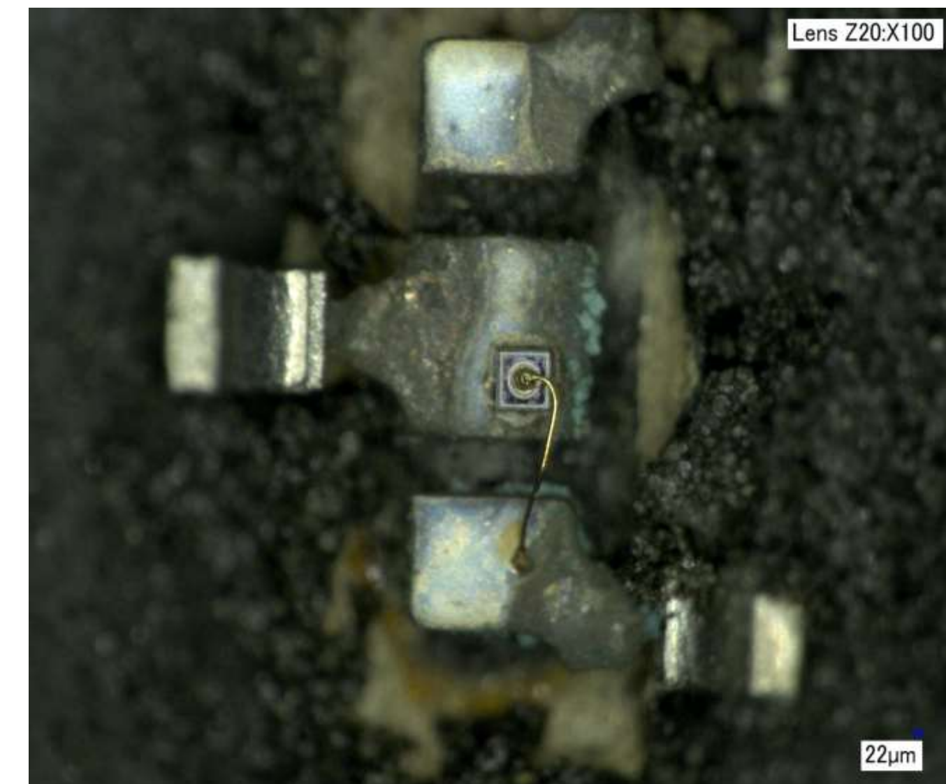
De-capped Infineon Diode
