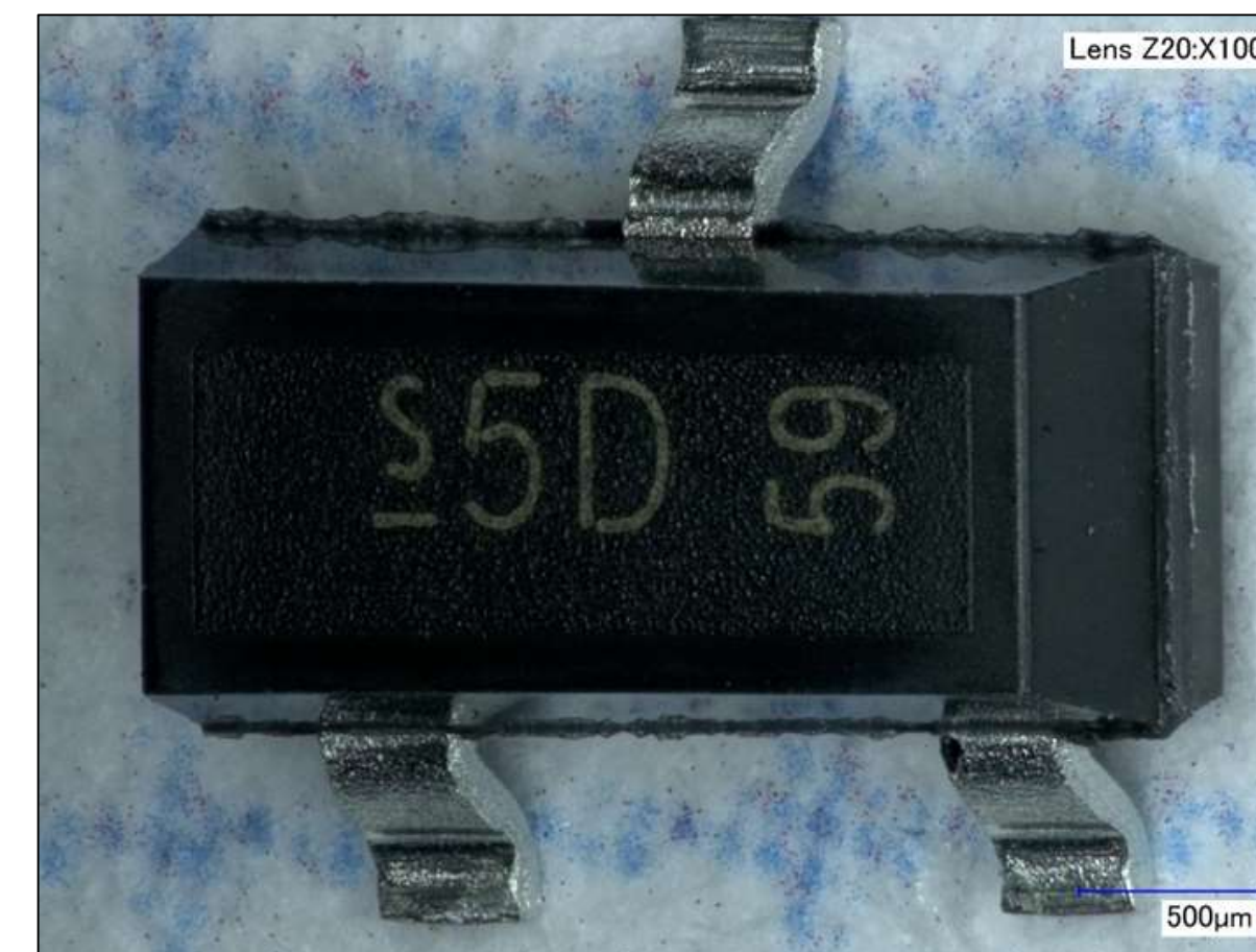
Examples of Infineon Diode Markings Following Solvent Tests (100X Magnification)
