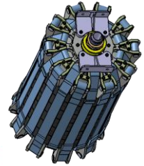
Step 7 Intergation in TAS of belt pin assy, retain system and test supports
