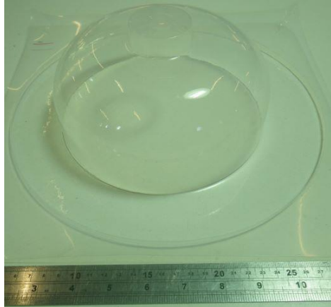
Vacuum formed endcap for open end (before trimming to size)
