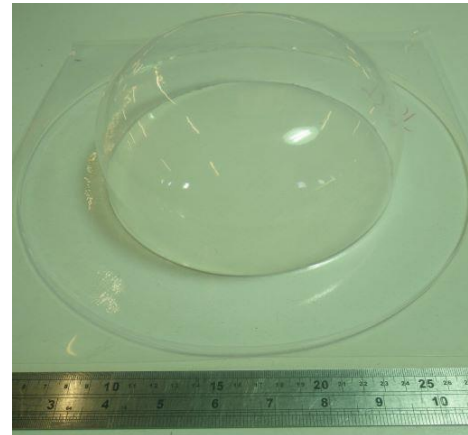
Vacuum formed endcap for closed end (before trimming to size)
