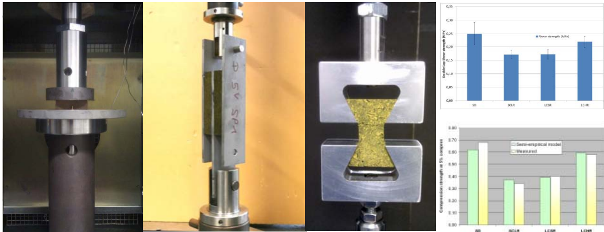
Figure 4: Measurement of mechanical properties at AAC (from left to right: compression, shear, tensile test apparatus, shear test results and compression results compared with semi-empirical model calculations)
