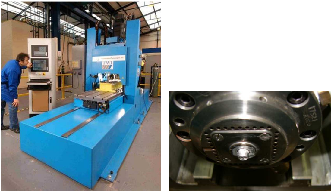
Figure 1 TWI's FSW machine and the FSW tool probe in the stationary shoulder welding head.
