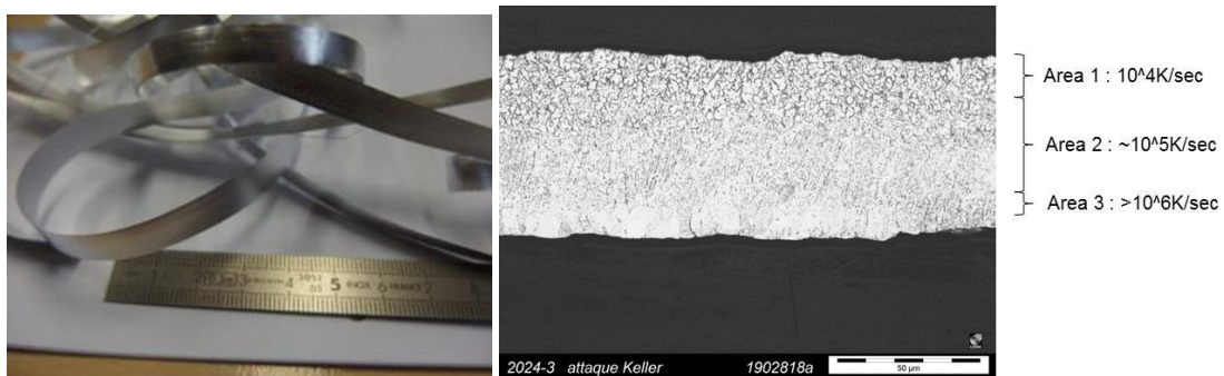
Figure 3: (left) view of a melt spun ribbon (right) cross section of the melt spun ribbon after etching. The solidification rates included in the picture are estimated from the size of the microstructure at different regions of the thickness.
