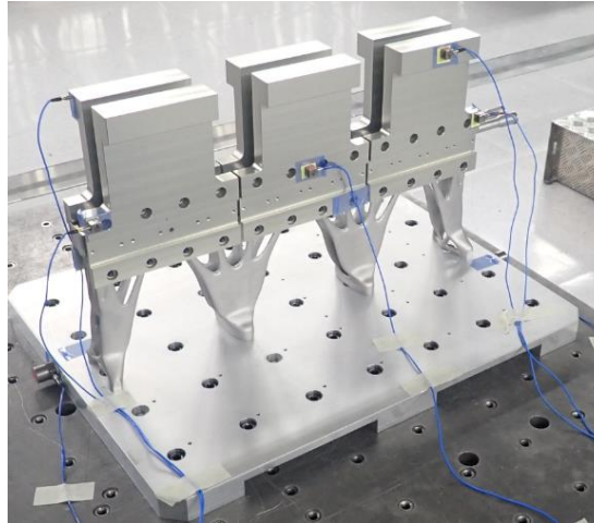
Equipped breadboard with dummies and accelerometers on vibration tool
