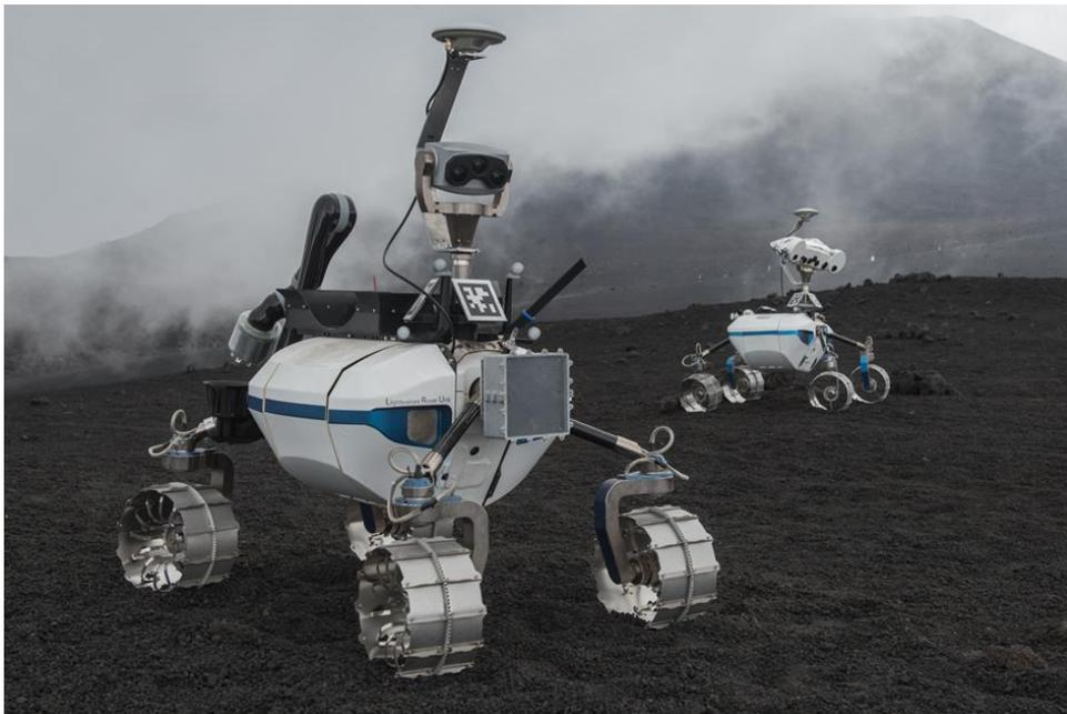
Figure 5: LRU Rover with JACO2 Arm and science cam operating in lunar analogue environment on Mt. Etna
