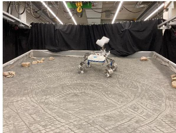
Figure 9: Gazebo simulation of the LRU in the PEL environment Figure 10: Real LRU rover in the PEL during test drives
