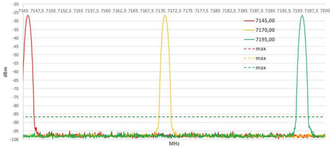
X band IF input 348.2/373.2/398.2MHz (Inverted)
