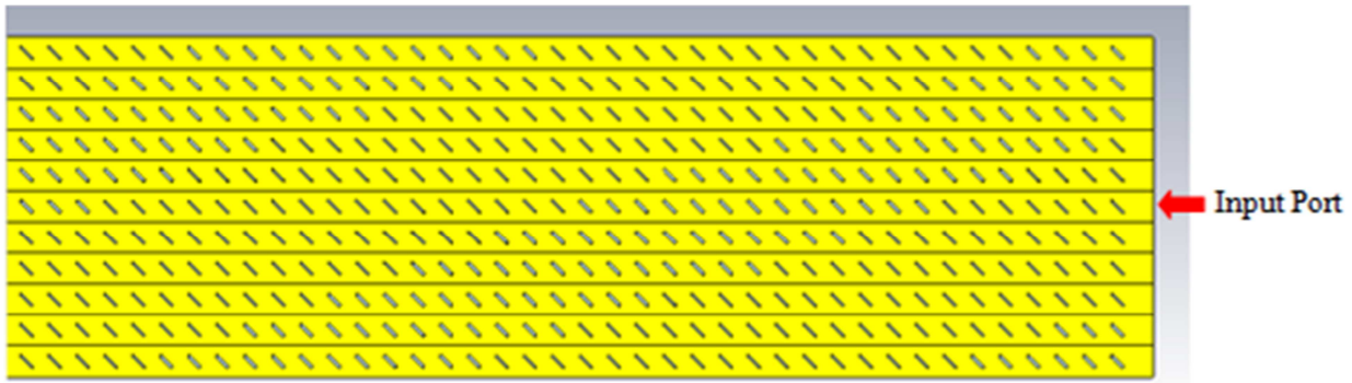
Figure 7.2: Leaky-wave planar array.
