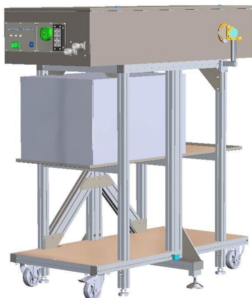
Figure 11 - 3D model design of the portable laser transmitter box
