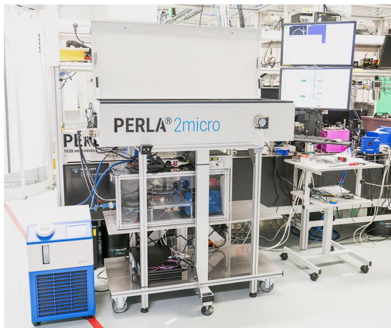
Figure 12 - The main laser transmitter as prepared at HiLASE laboratory
