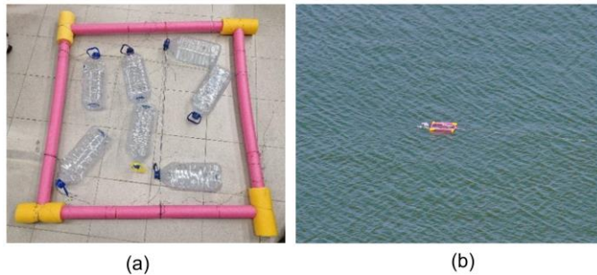
Figure 21: Example of targets used in the S4 scenario. (a) Detail of the square frame made of Polyurethane foam and attached bottles. (b) The target on the water, where a capillary wave pattern is visible.
