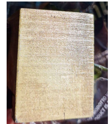
Metallized specimen in PEEK-CF and ULTEM
